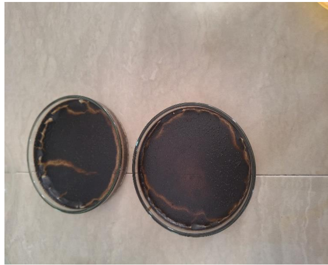
Fig. 2. The preparation of graphene oxide from graphite powder
