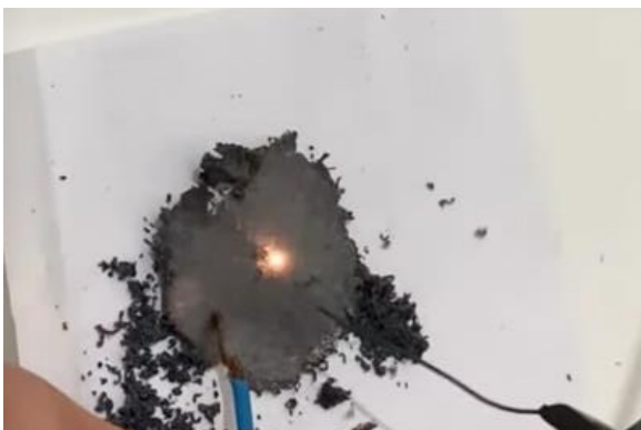
Fig. 5. Electrical conductivity of GO in a applied simple setup for energy harvesting
