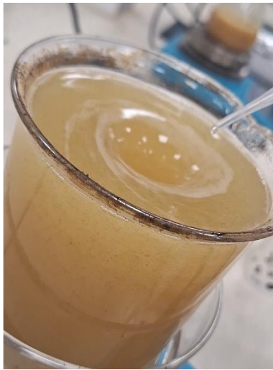
Fig. 2. The preparation of graphene oxide from graphite powder
