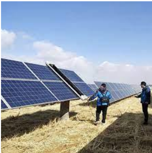
Fig. 2. A semi-automatic solar pv panel washing/ cleaning machine.
