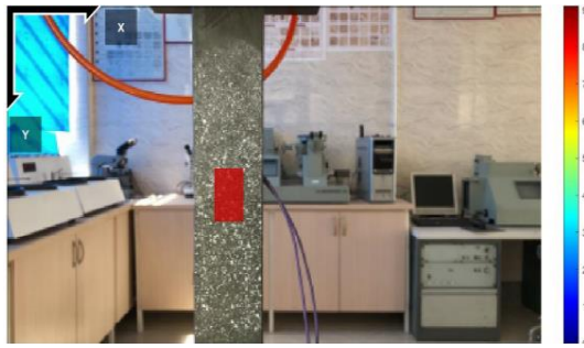
Fig. 11. Image of DIC method under applied loads.
